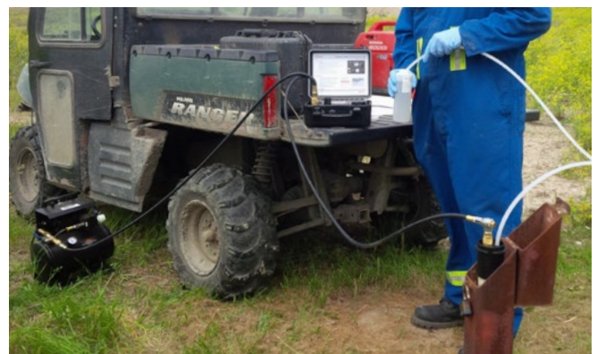
Sampling with a Dedicated Bladder Pump using Portable, Rugged, Easy-to-use, Compressor and Controller
