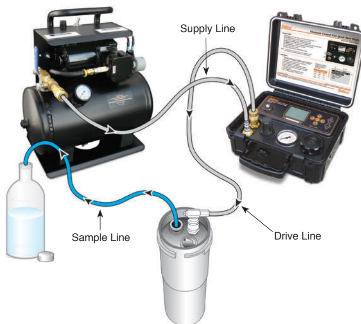
Pumping Setup with 125 psi Model 464 Electronic Pump Control Unit and 12 Volt Compressor
